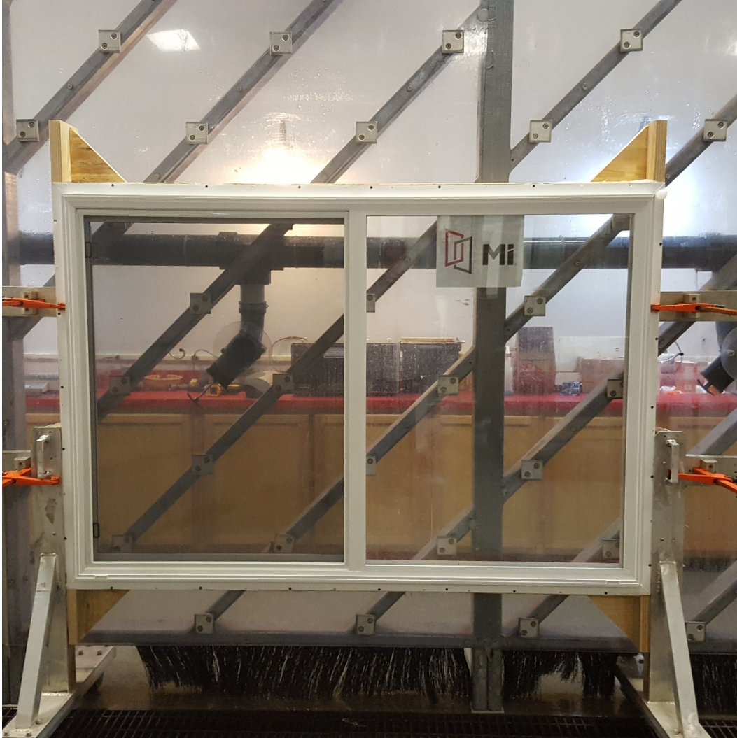
Photo 1 Series 1630 Horizontal Sliding Window (fin installation)
